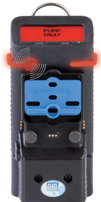
G460 with pump activated: - Sensor cover UP - Diffusion inlets covered
