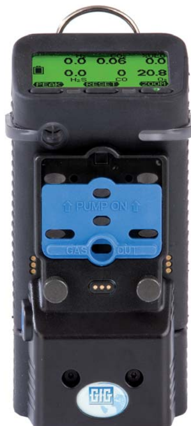
G460 with pump de-activated: - Sensor cover DOWN - Diffusion inlets open
