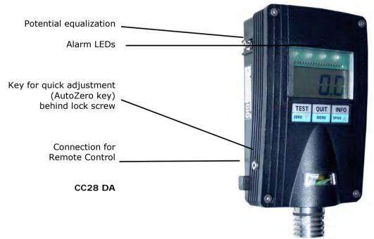
The type label shows the transmitter type. The sensor enclosure includes the sensor and the sensor card, which carries the components for the sensor circuitry. For adjustment of electrical zeropoint and sensitivity you can use either the built-in display or the remote control RC2. A secured key at the left side of the transmitter allows a quick zero setting. The electronics on the main p.c.board converts the sensor signal into a linear output signal of 4 .. 20 mA.
