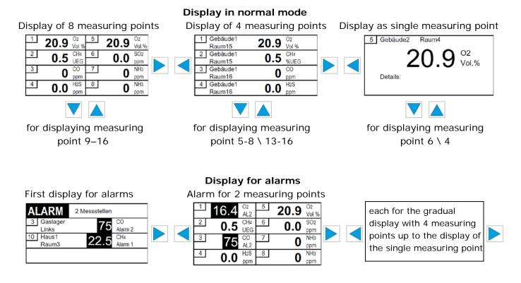
The display is backlit; the light intensity can be increased via any control button. In the event of a gas alarm or faults, the display lighting is automatically activated with a red background.
