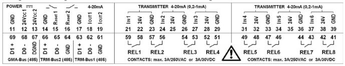
The top terminal assignment applies to the GMA200-MT6 and the bottom terminal assignment applies to the GMA200-MT16.
