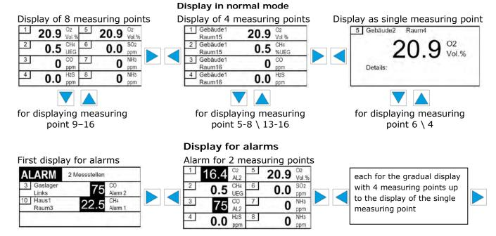
The graphical display is backlit; the light intensity can be increased via any control button. In the event of a gas alarm or faults, the display lighting is automatically activated with a red background.
