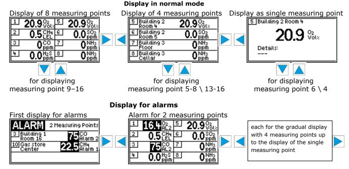
The graphical display is backlit; the light intensity can be increased via any control button. In the event of a gas alarm or faults, the display lighting is automatically activated with a red background.
