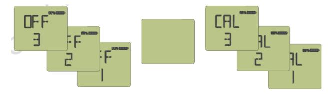
The detector will first automatically zero the sensors at the current baseline reading. Then the detector will prompt to "APPLY GAS":
