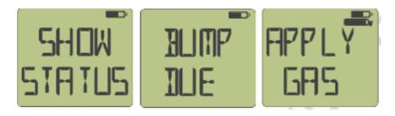
The detector will flash between "BUMP DUE" and "APPLY GAS". Apply gas to the unit at a flow rate of 0.25 to 0.5LPM using the calibration cap provided. Once all sensors have gone into alarm, the unit will return to normal operation (in alarm) and the bump due date will be reset.
