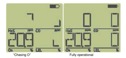
Once all sensors have completed the warm up sequence the detector is ready to detect all gases.
